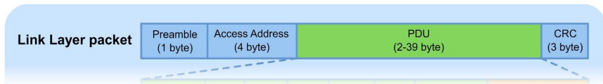
Figure 2-E: Link Layer packet structure
